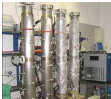
Laboratory set-up for testing the elimination of trace organics and pathogenic microorganisms during soil passage
