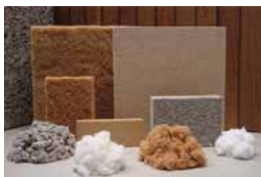
Insulation with renewable primary products (hemp, wood and cellulose fiber)
